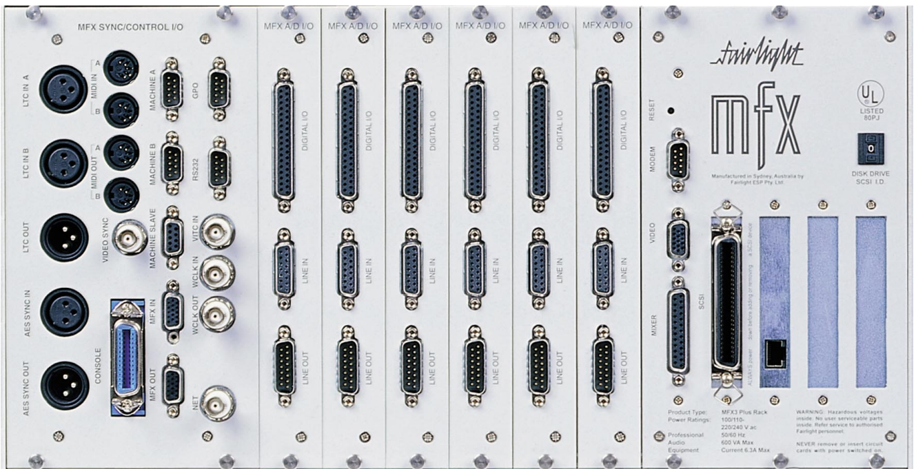
Mainframe Rear Panel - Detail of Connections
